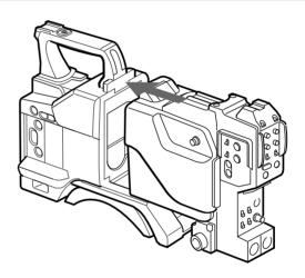
**4** Tighten the two screws (M4  $\times$  12) in the figure.
